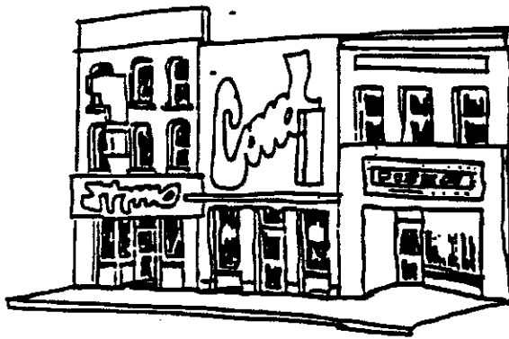
INFILLED STOREFRONT WINDOWS
